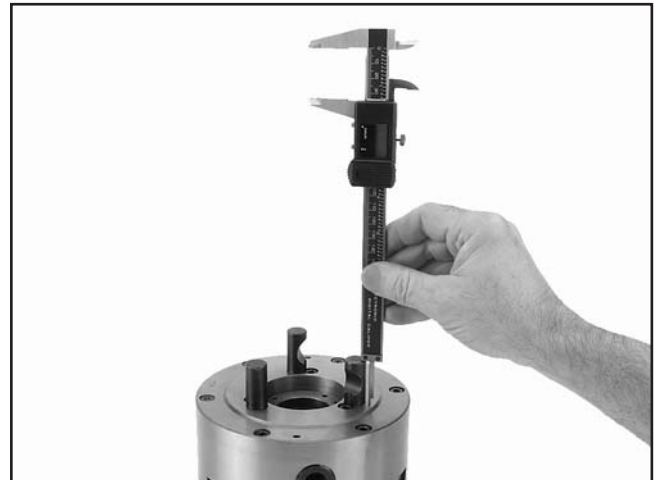
Figure 23. Measuring height of cam-lock studs.
