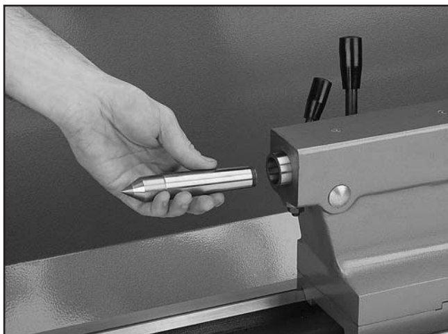
Figure 34. Inserting a dead center in a tailstock.
