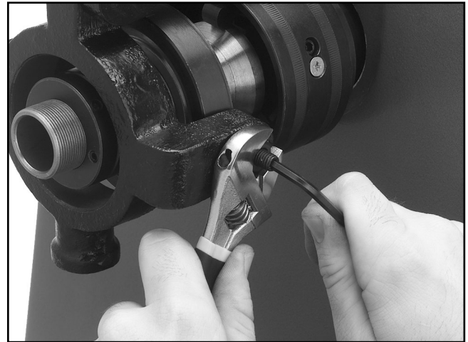
Figure 10. Tightening yoke setscrews.
