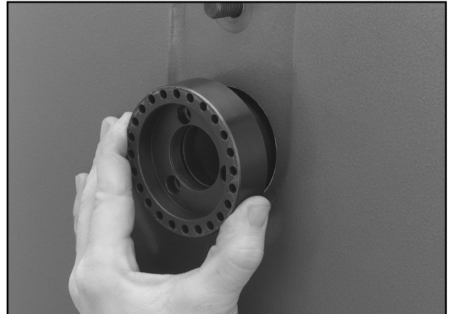
Figure 4. Installing hub adapter.
