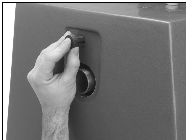
Figure 1. Lathe cover removal.
