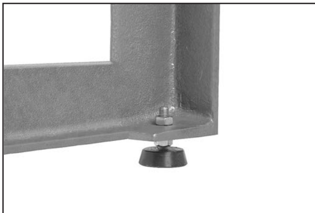
Figure 14. Machine feet installed.
