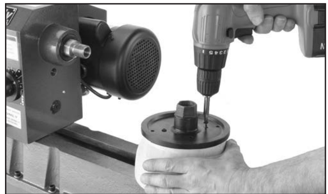
Figure 37. Typical attachment of faceplate to workpiece.
