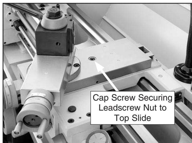
Figure 99. Location of cap screw that secures the leadscrew nut.
