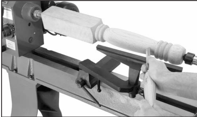
Figure 39. Typical spindle turning operation.
