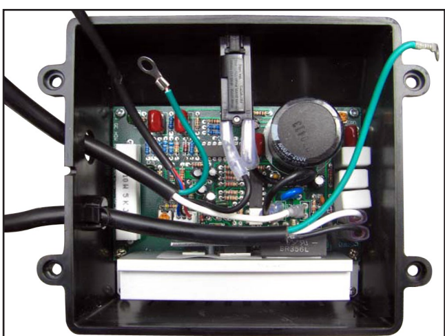
Figure 52. Motor control box wiring.
