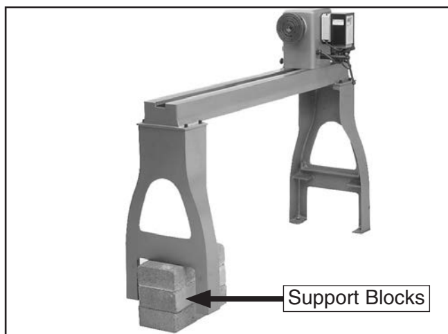
Figure 13. Example of supporting one end of lathe in preparation for installing the machine feet.
