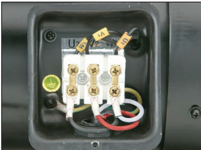
Figure 59. Model G0632 motor junction box wiring.
