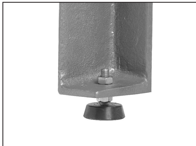
Figure 14. Machine feet installed.
