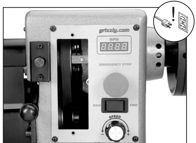
Figure 32. Belt access panel removed.
