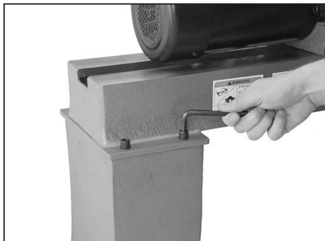
Figure 12. Securing lathe assembly to supporting legs.
