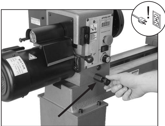
Figure 21. Pulling out the swivel pin.
