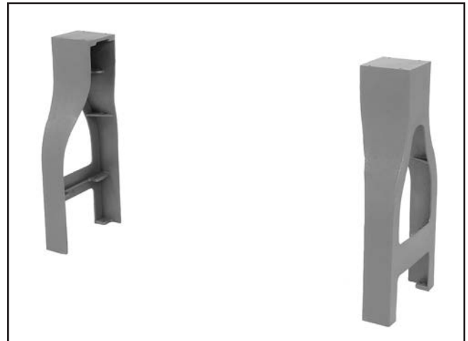
Figure 11. Stand legs approximately 47" apart to prepare for mounting the lathe.
