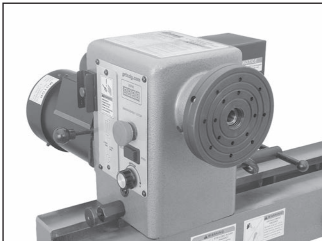
Figure 49. Headstock set at 90°.
