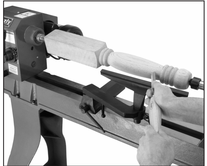
Figure 20. Typical spindle turning operation.
