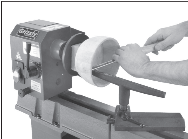
Figure 24. Typical faceplate turning operation.
