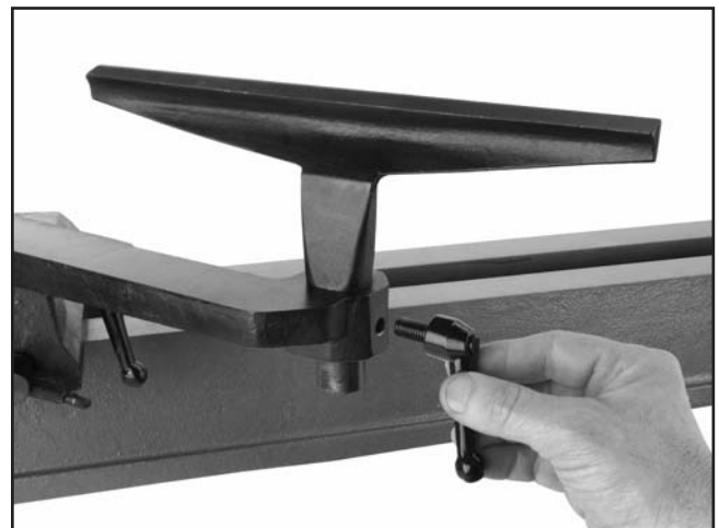
Figure 8. Installing handle into tool rest.
