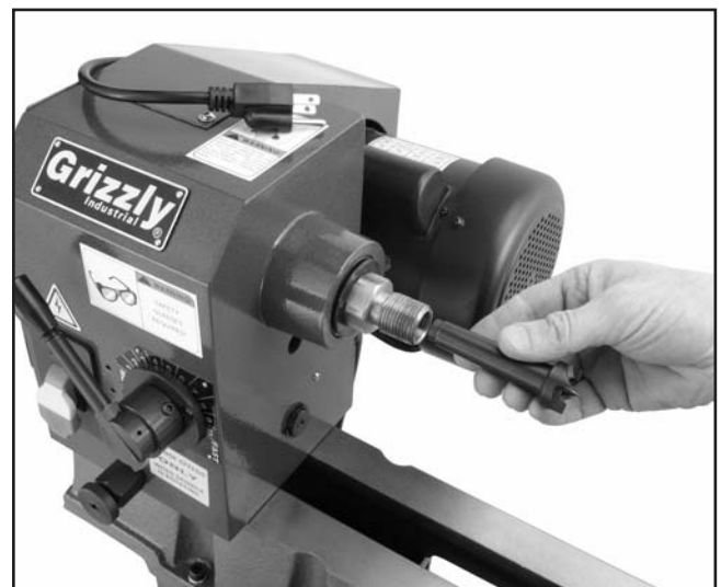
Figure 15. Inserting spur center into spindle.
