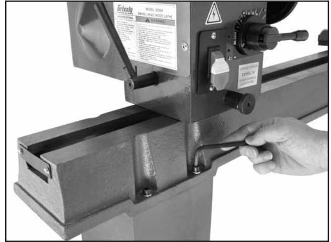
Figure 7. Securing lathe to stand legs.
