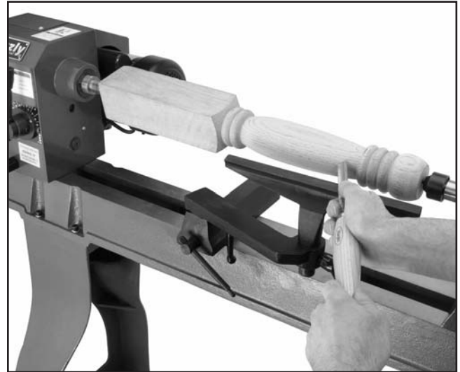
Figure 24. Typical spindle turning operation.
