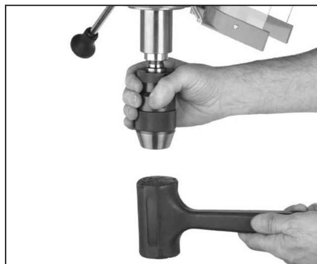
Figure 17. Seating arbor and chuck into spindle.
