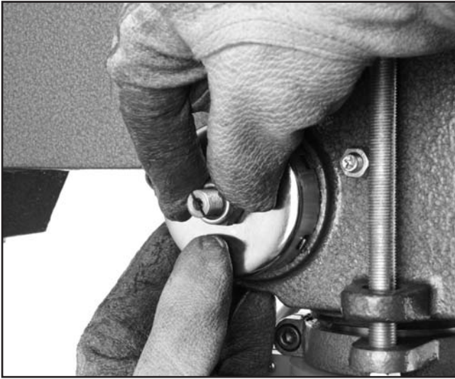
Figure 44. Loosening cover and jam nut.
