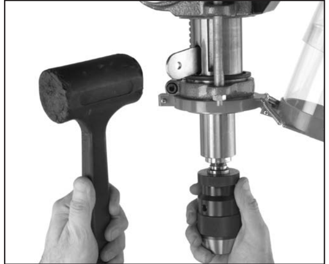
Figure 33. Using drift key to remove arbor.
