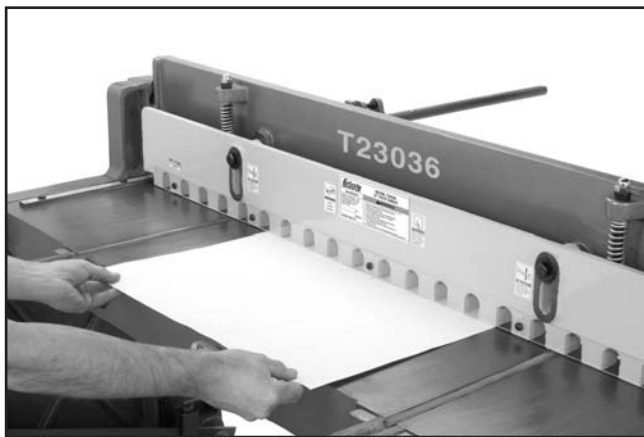
Figure 26. Example of a paper shear test.
