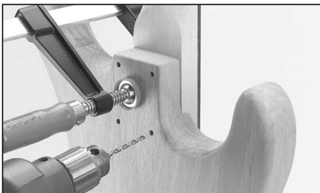
Figure 14. Drilling the screw holes.
