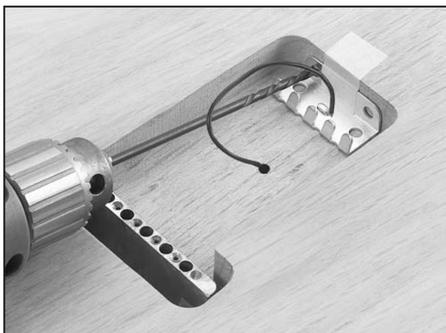
Figure 24. Drilling the spring hanger mounting holes.
