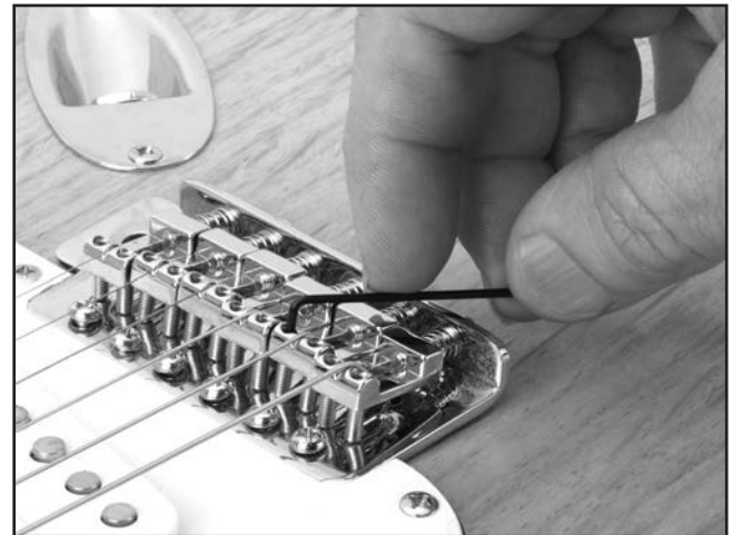
Figure 38. Adjusting string height.
