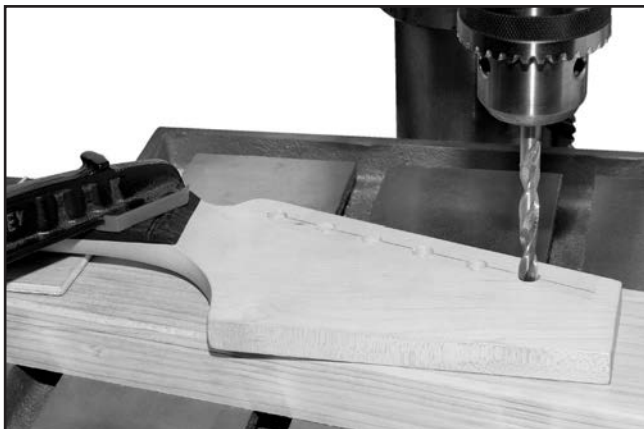
Figure 10. Drilling the pegholes.
