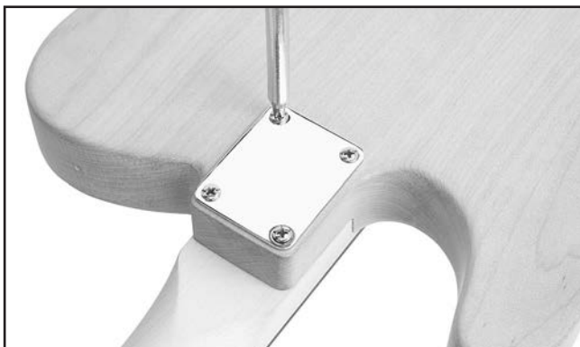
Figure 20. Fastening neck to body.
