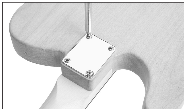
Figure 20. Fastening neck to body.
