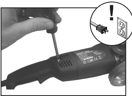
Figure 16. Removing the T10494 and T10495 brush covers.
