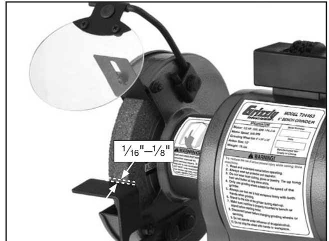
Figure 12. Model T24463 tool rest gap.
