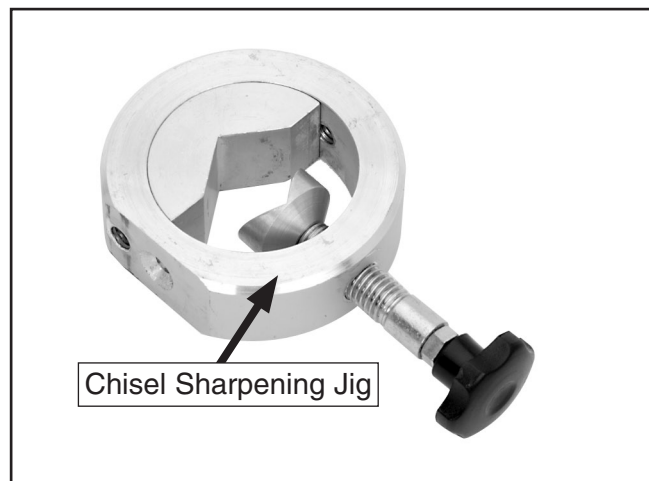
Figure 9. Hollow chisel jig assembly.
