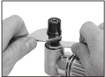
Figure 2. Loosening the collet.
