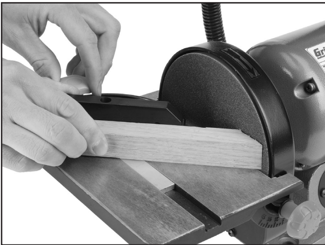
Figure 12. Disc sanding with a miter gauge.
