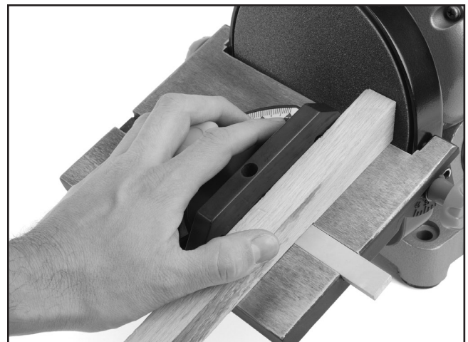
Figure 13. Mitering with the table angled.
