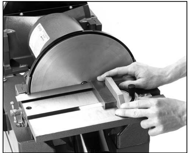
Figure 7. Squaring miter gage to disc.
