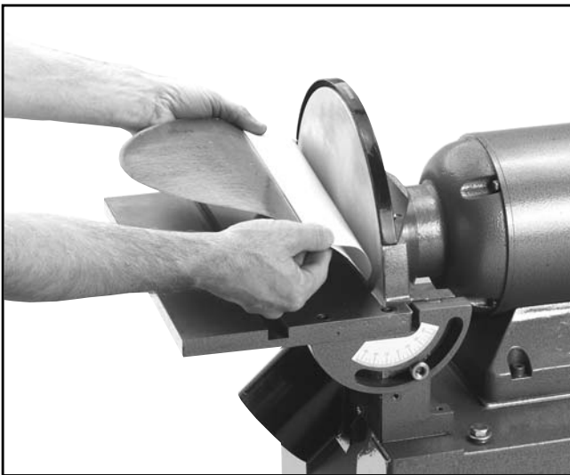
Figure 4. Sandpaper being slipped between the disc and table.
