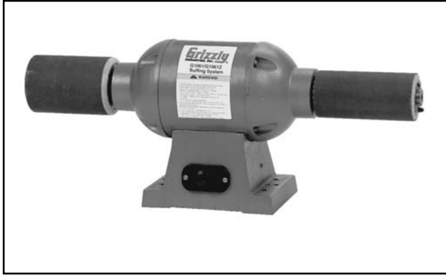
Figure 3. Sanding drums installed.
