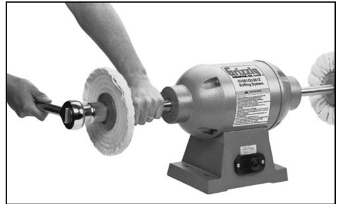
Figure 4. Buffing wheel loosening/tightening procedure.
