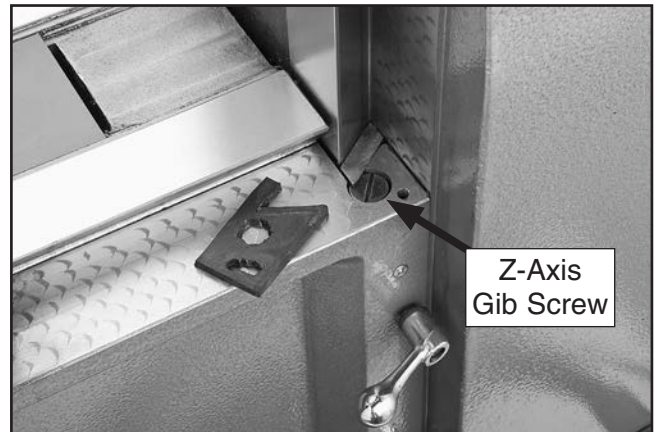
Figure 82. Location of Z-axis gib adjustment screw.
