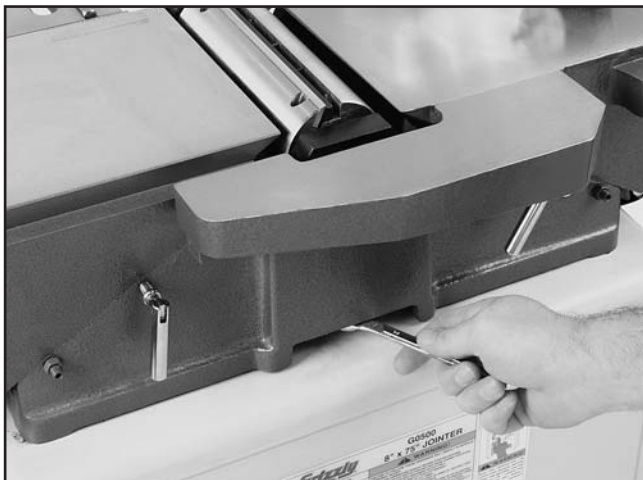
Figure 4. Example of removing nut and lock washer on bearing block stud.
