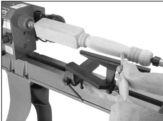
Figure 31. Typical spindle turning operation.
