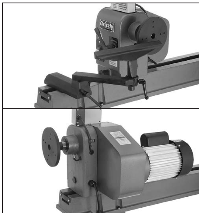
Figure 19. Head set at 90^\circ and 180^\circ .
