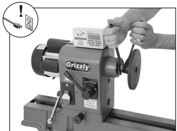
Figure 26. Tightening the faceplate onto the spindle.
