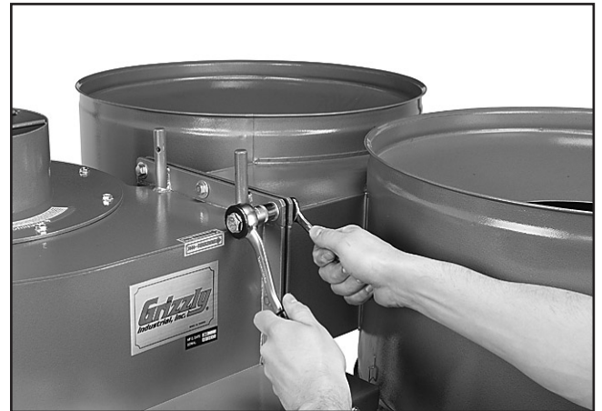
Figure 7. Mounting collectors to motor/fan assembly.
