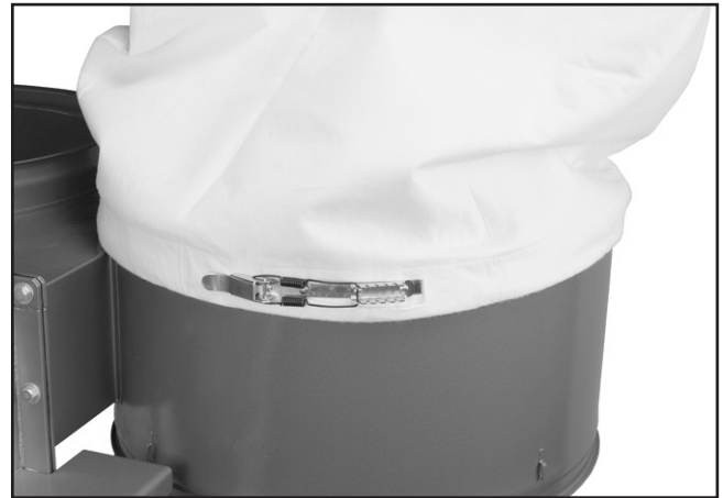
Figure 9. Fitting bag onto collector.
