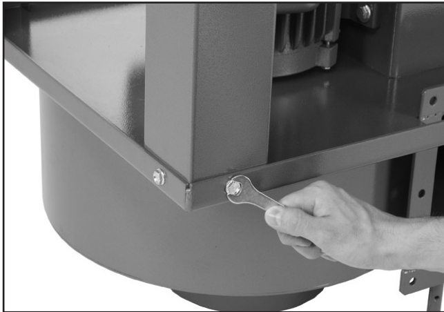
Figure 5. Attaching legs to motor/fan assembly.
