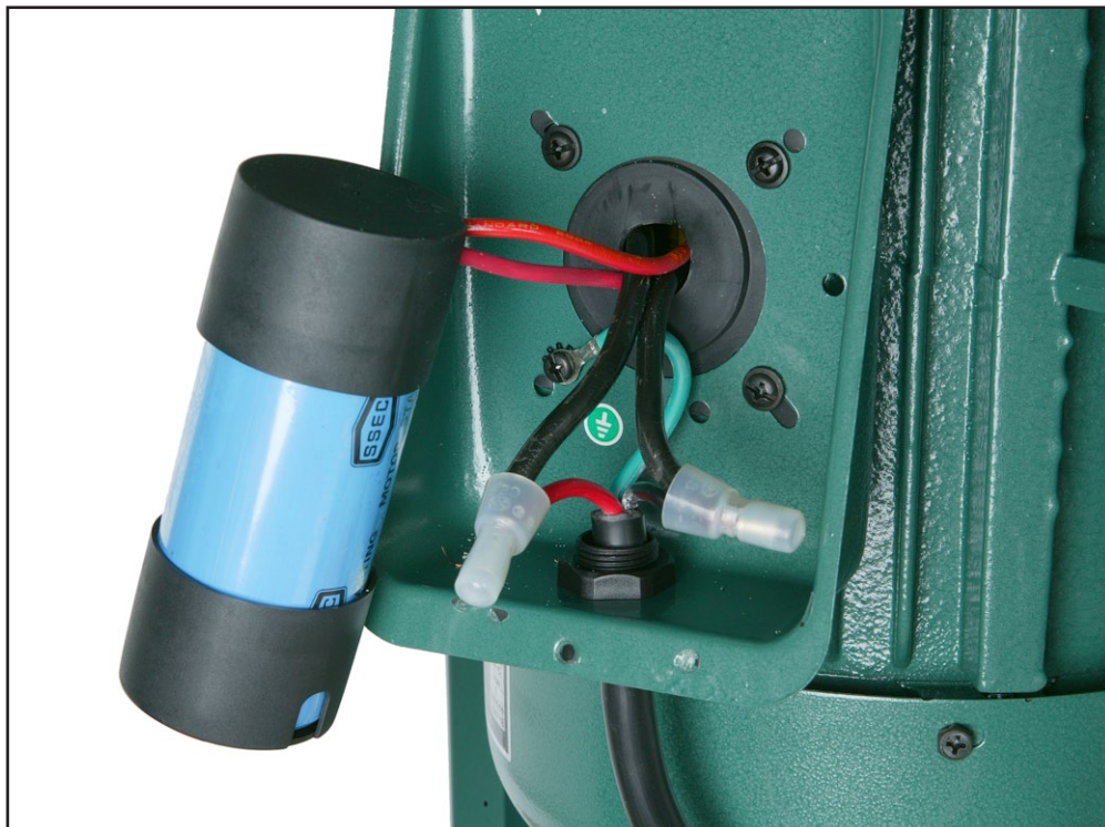
Figure 32. Model G5954 Junction Box Wiring.
