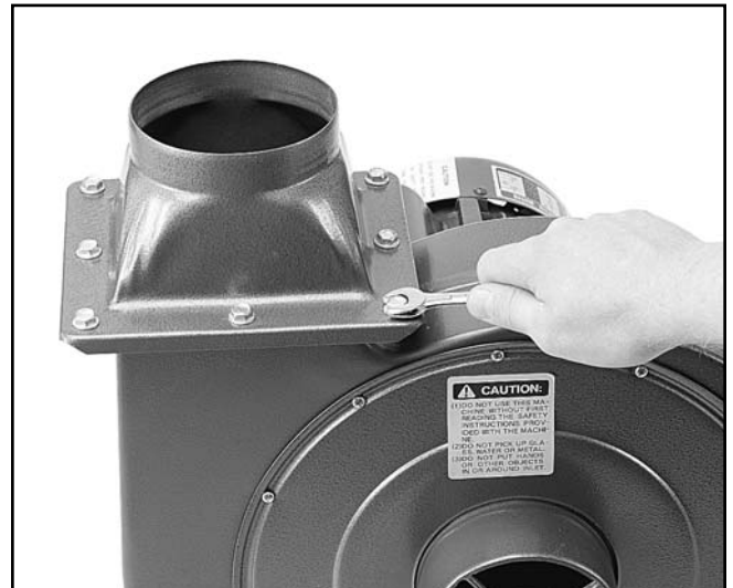
Figure 4. Mounting outlet to collector body.
