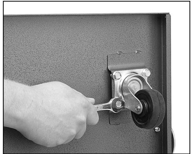
Figure 2. Mounting casters to base.
