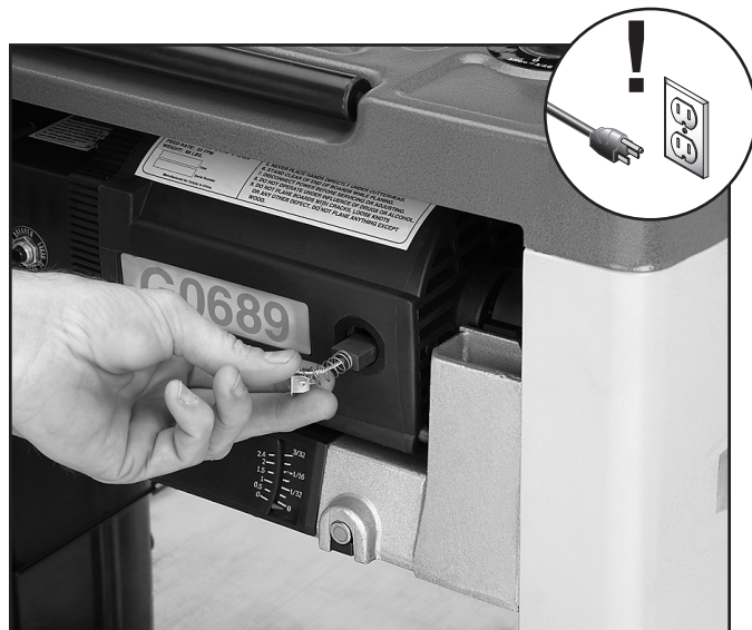
Figure 34. Brush holder location (another brush is located on the other side of the motor from the one shown in this picture).
