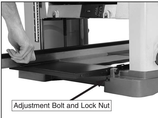
Figure 40. Aligning extension wings.
