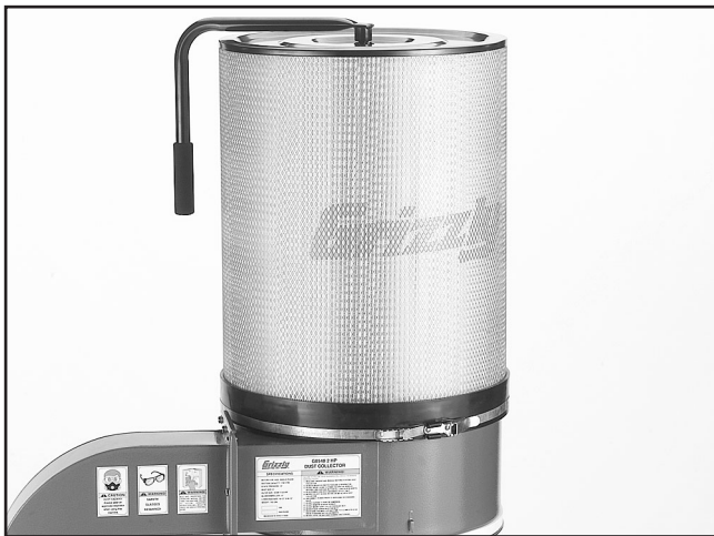
Figure 17. Installed and secured canister filter.
