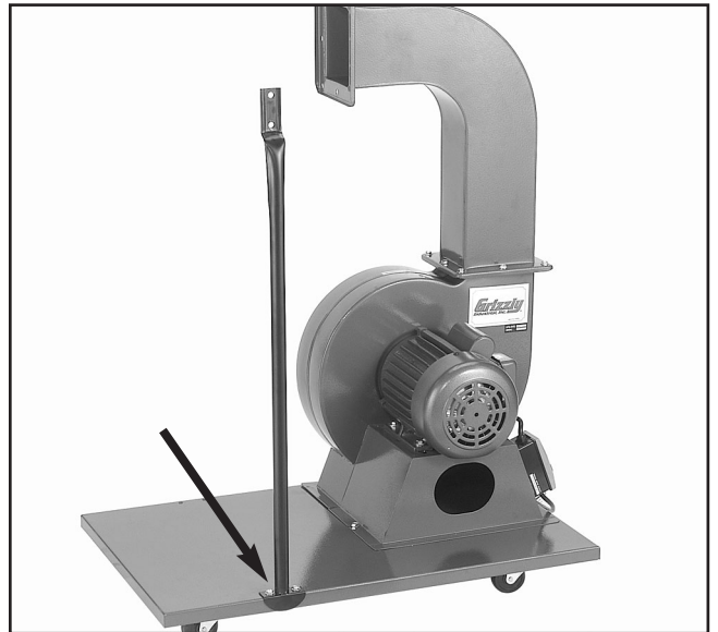
Figure 11. Canister support attached to base.
