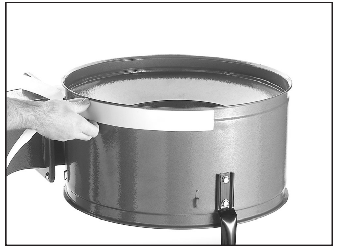
Figure 14. Installing wide foam strip.
