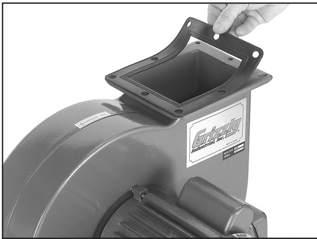
Figure 9. Placing rubber gasket over outlet.
