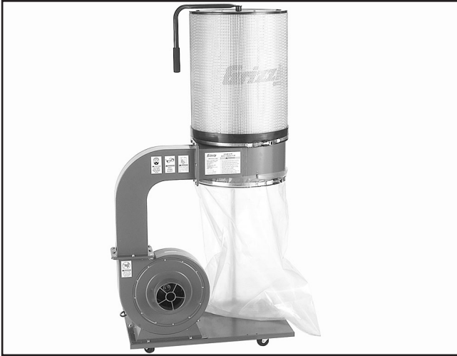
Figure 19. Lower collection bag installed.
