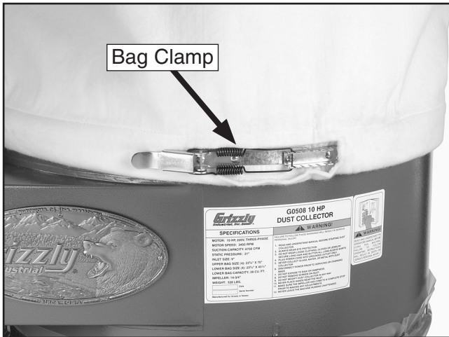
Figure 14. Upper filter bag secured to collector.
