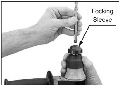
Figure 3. Inserting the bit into hammer drill.
