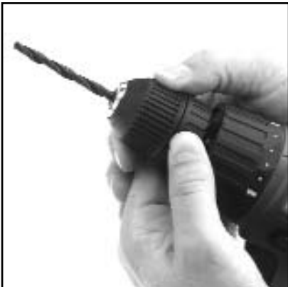
Fig 1. Inserting bits into the chuck.
