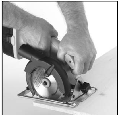
Fig 9. Proper Holding Grip.
