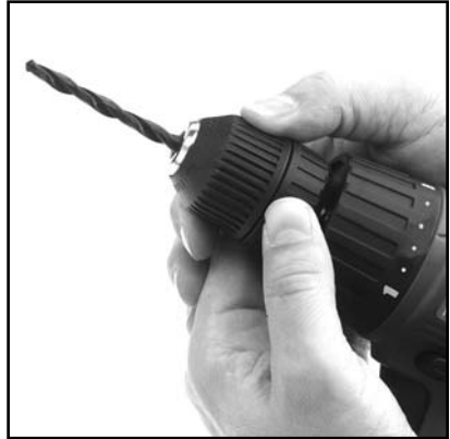
Fig 2. Inserting bits into the chuck.
