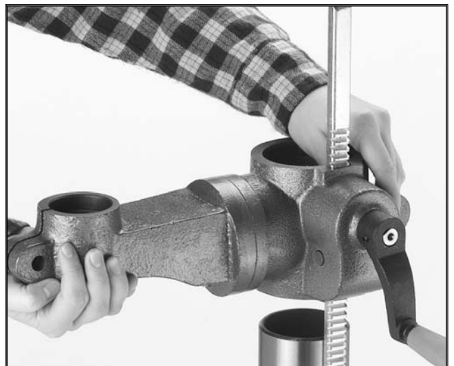
Figure 6. Rack orientation (G7946 shown).
