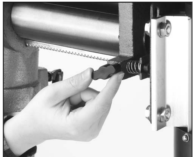
Figure 10. Loosening the lock knob.
