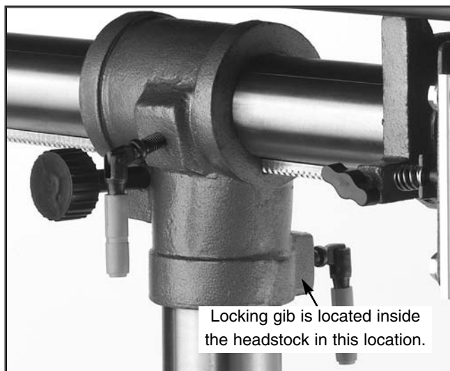
Figure 8. Lock Handles and gib location.
