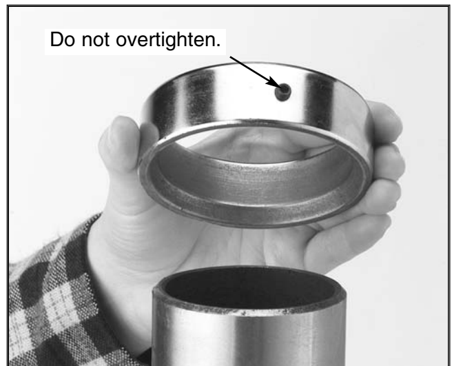
Figure 7. Inside bevel in the correct position.
