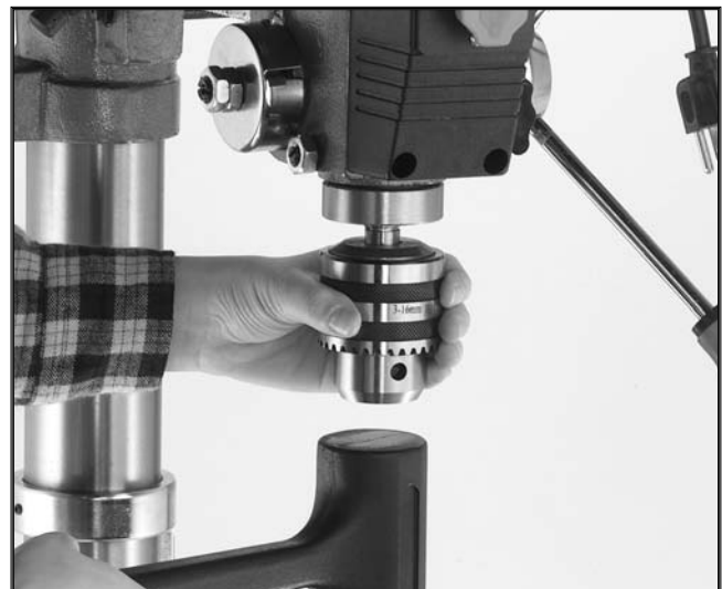
Figure 9. Seating chuck into spindle. (Note retracted jaws.)
