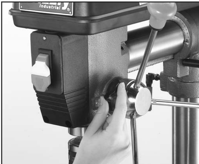
Figure 11. Loosening collar lock knob.
