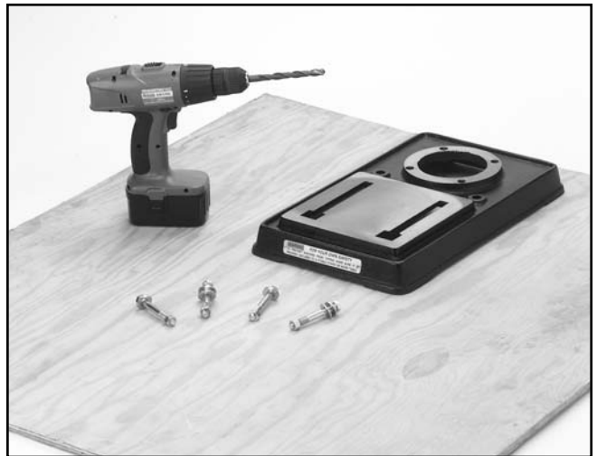
Figure 3. Attaching plywood sub-base.
