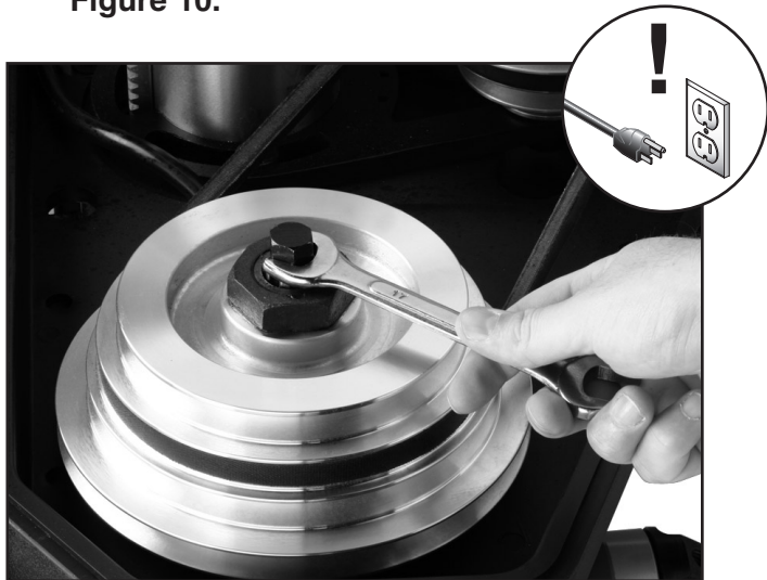
Figure 10. Turning the drawbar nut.
