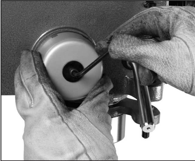
Figure 29. Loosening cover and cap screw.
