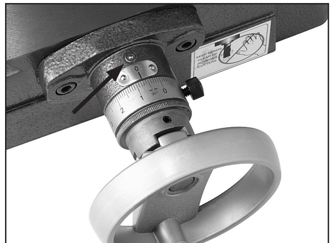
Figure 26. Handwheel oiling location.
