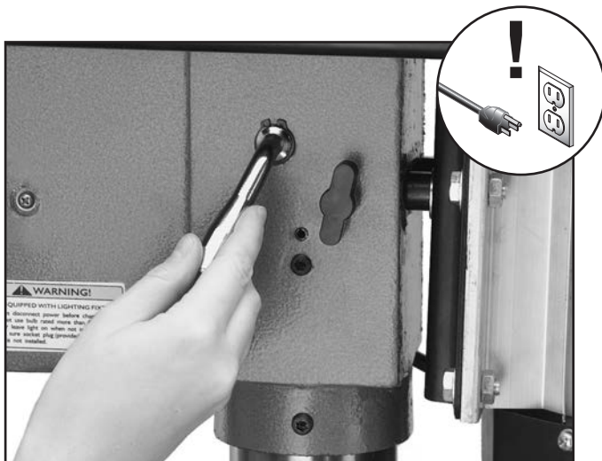
Figure 27. Using the belt tension lever.
