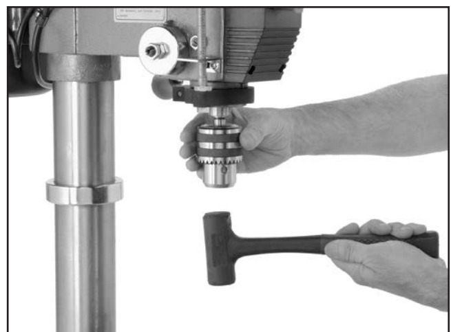
Figure 16. Seating arbor and chuck into spindle.
