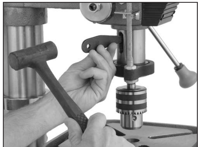
Figure 33. Using drift key to remove arbor.
