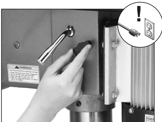
Figure 26. Loosening lock knob (both sides).
