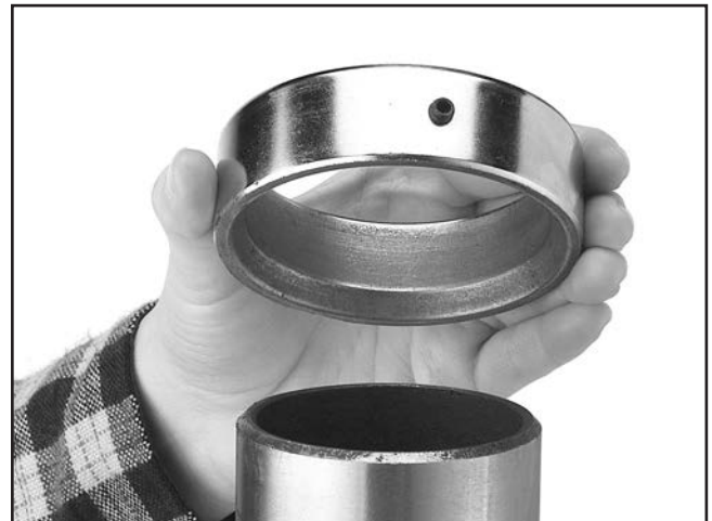
Figure 10. Correct column ring orientation.
