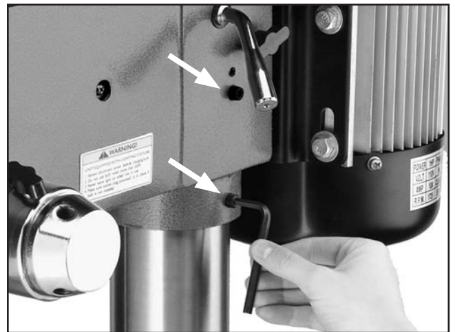
Figure 13. Securing headstock to column.
