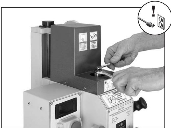
Figure 28. Snugging the drawbar.
