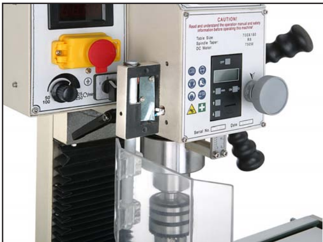
Figure 62. Chip guard limit switch.
