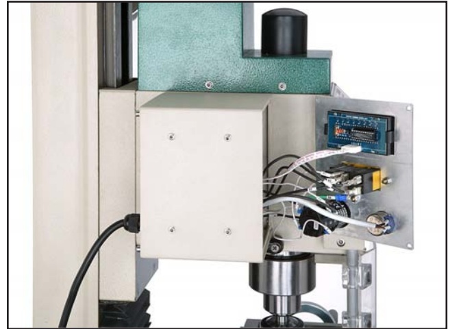
Figure 63. Control panel wiring.
