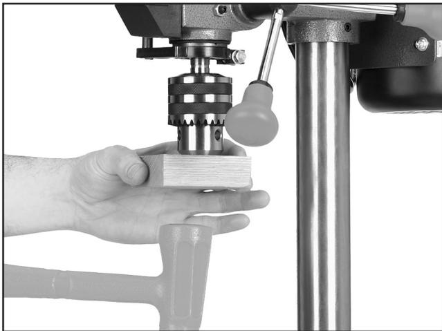
**Figure 28.** Seating the chuck on the arbor.
