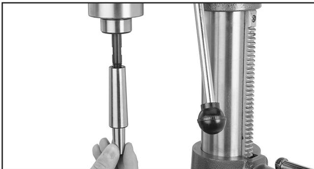
**Figure 24.** Inserting tooling into spindle.
