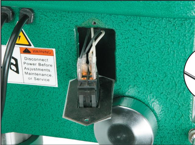
Figure 50. Power switch assembly.
