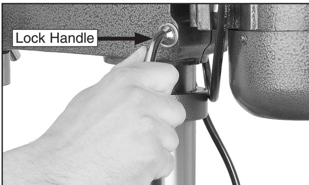
**Figure 11.** Securing headstock to column.
