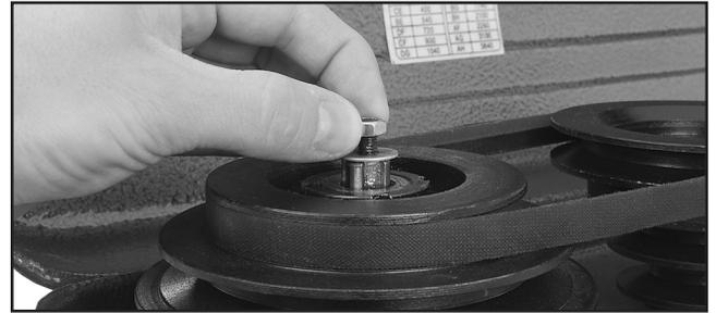
**Figure 25.** Tightening nut on drawbar.
