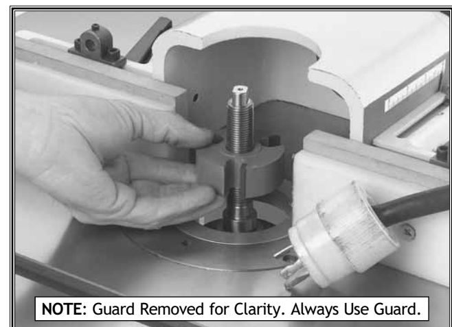
Figure 6. Unplug the shaper whenever making adjustments or changing cutters.
