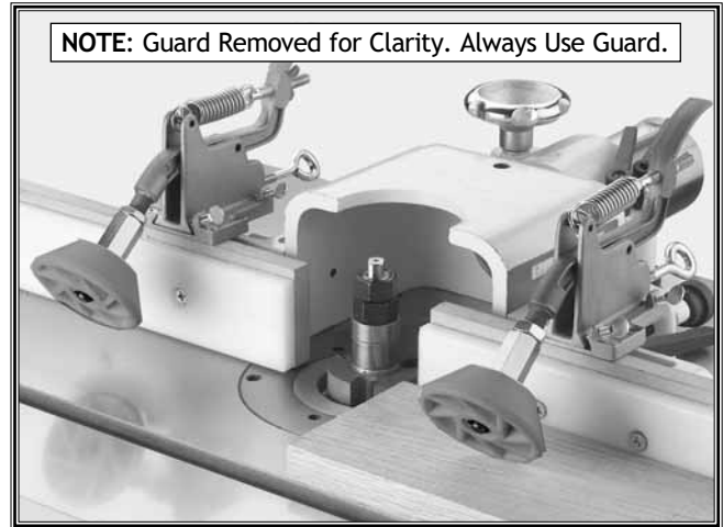
Figure 4. Use SHOP FOX® BOARD BUDDIES® for holding down the workpiece.
