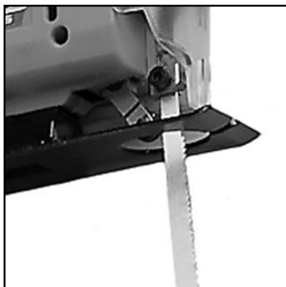
Fig 3. Jig saw blade installation.
