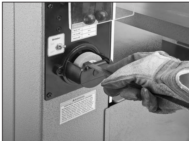
Figure 43. Using the grinder to square up the blade end.
