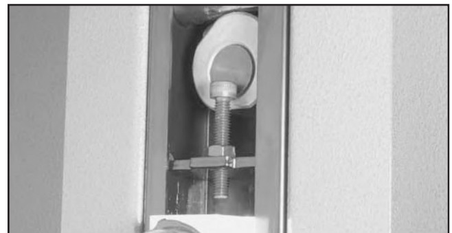
Figure 7. Tension adjustment assembly locations (top wheel removed for clarity).
