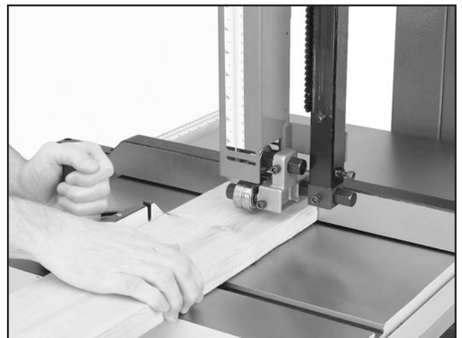
Figure 44. Crosscutting with miter gauge.
