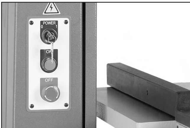
Figure 38. G0514X/G0514X3 START/STOP switch.
