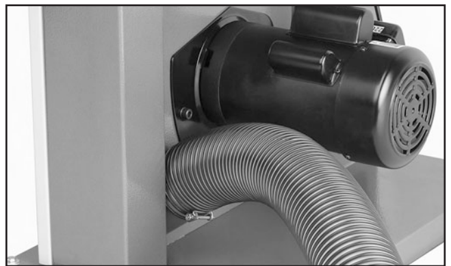
Figure 21. Dust hose attached to dust port.
