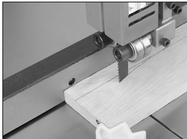
Figure 41. Blade leading away from line of cut.
