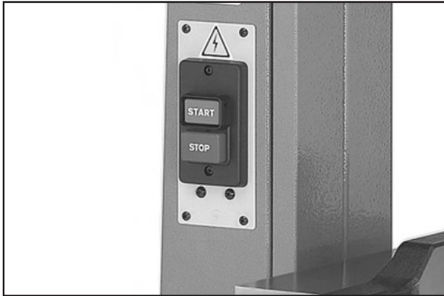
Figure 37. G0513X START/STOP switch.
