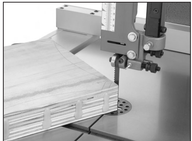
Figure 46. Typical stacked cut.
