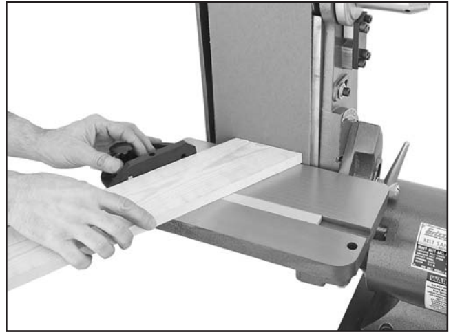
Figure 39. Example of vertical miter sanding.
