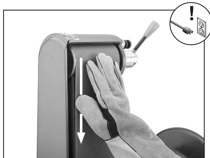
Figure 23. Rotating the sanding belt to check belt tracking.
