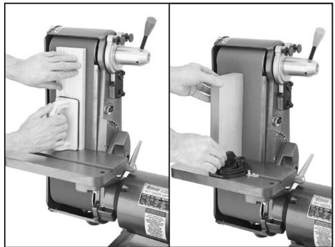
Figure 40. Examples of vertical face and edge sanding.
