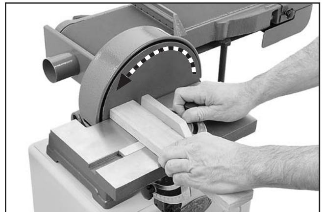
Figure 32. Example photo of 90° disc sanding.
