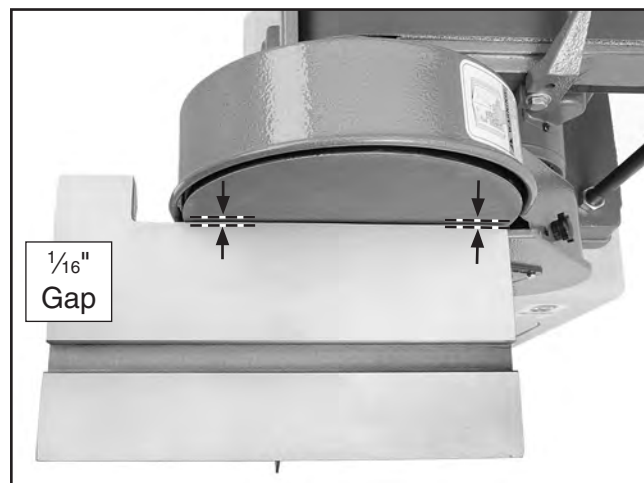
Figure 35. Correct distance between disc and work table.
