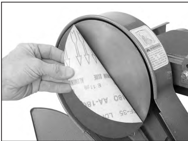
Figure 30. Installing sanding disc onto cast iron plate.
