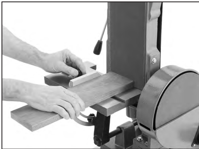
Figure 72. Example of end grain sanding.
