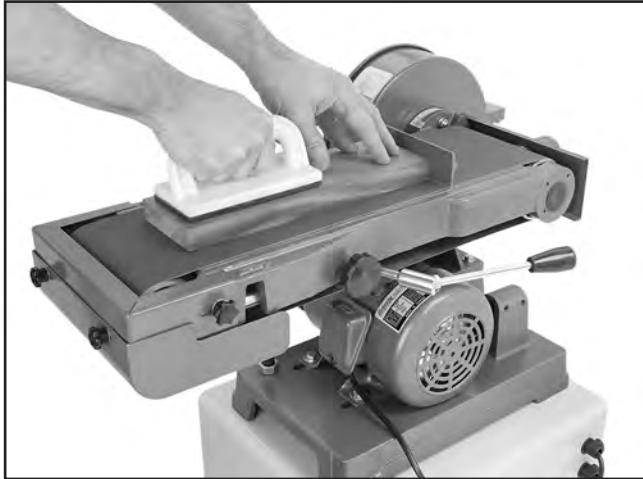
Figure 57. Sanding workpiece in horizontal position.
