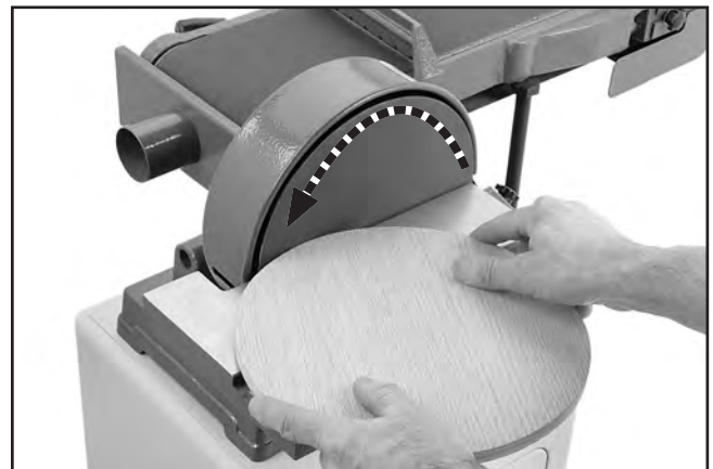
Figure 63. Example of sanding round workpiece.
