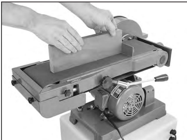
Figure 58. Sanding edge of workpiece in horizontal position.
