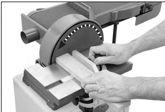
Figure 60. Example of 90° disc sanding.
