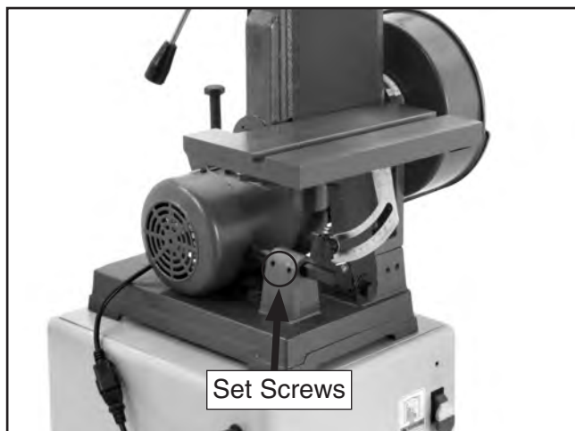
Figure 55. Location for removing work table assembly.
