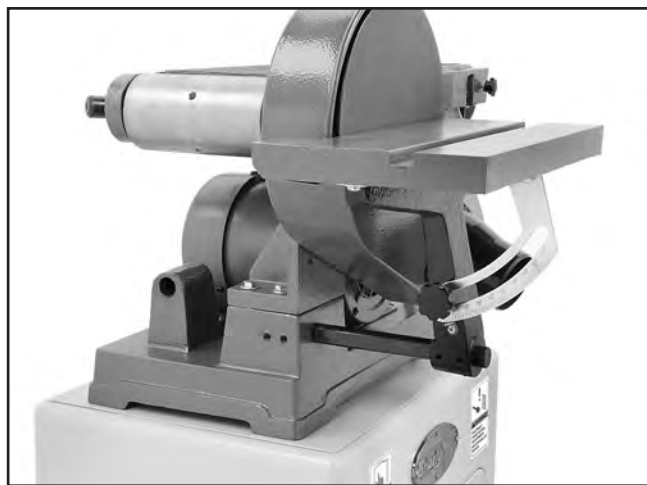
Figure 34. Installing work table onto table support rod.
