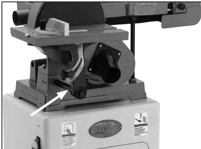
Figure 86. Table support rod lubrication.
