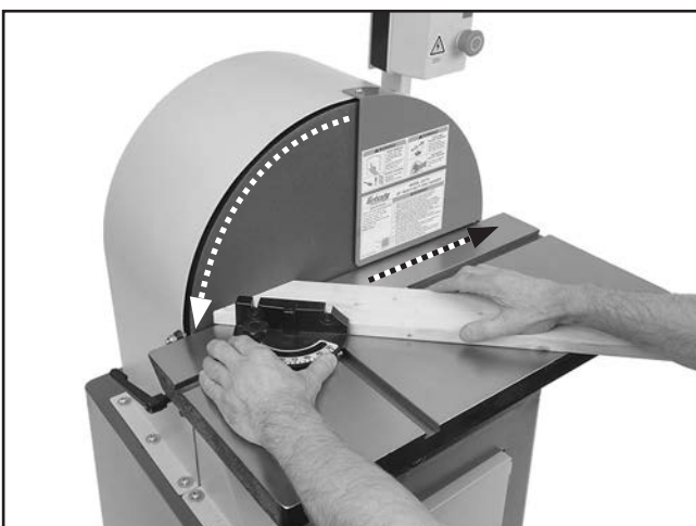
Figure 12. Example of angle sanding.
