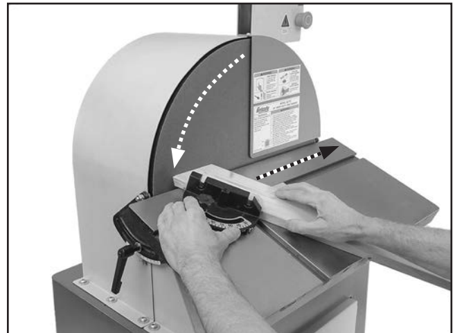
Figure 13. Example of sanding with table tilted.
