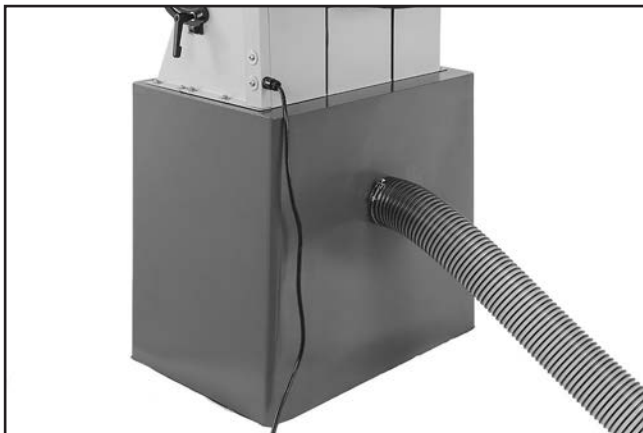
Figure 8. Dust hose attached to dust port.
