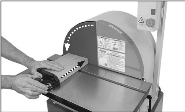
Figure 10. Example of Y-axis sanding.
