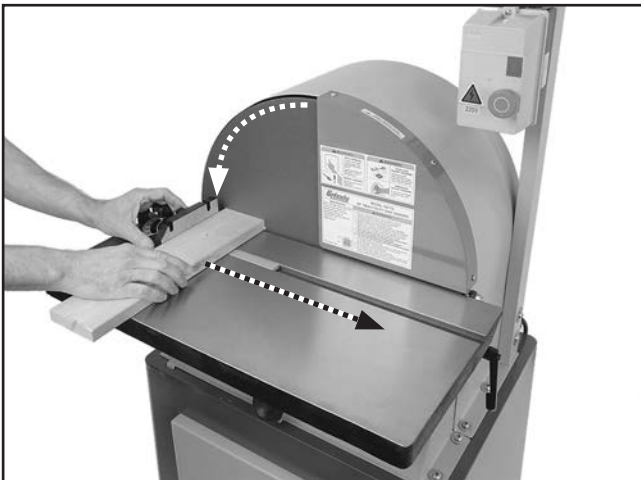
Figure 11. Example of X-axis sanding.
