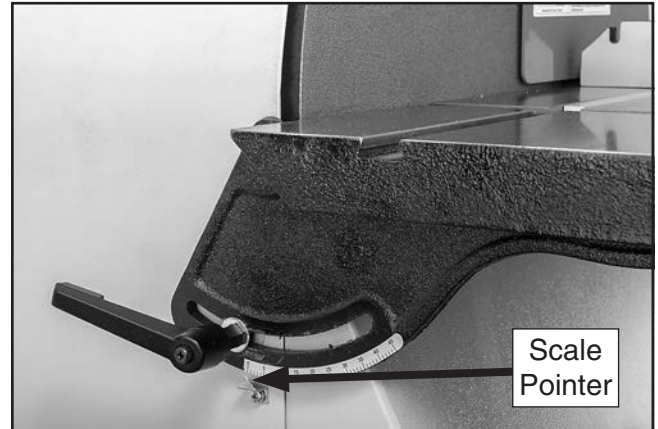
Figure 27. Scale pointer screw location.
