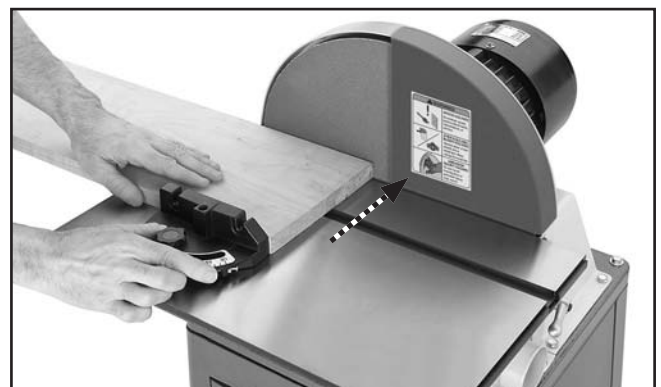
Figure 16. Example of Y-axis sanding.
