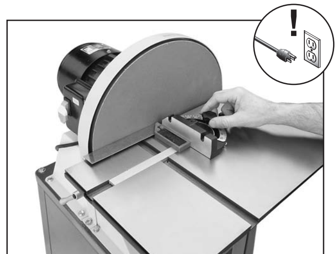
Figure 25. Squaring miter gauge to disc.
