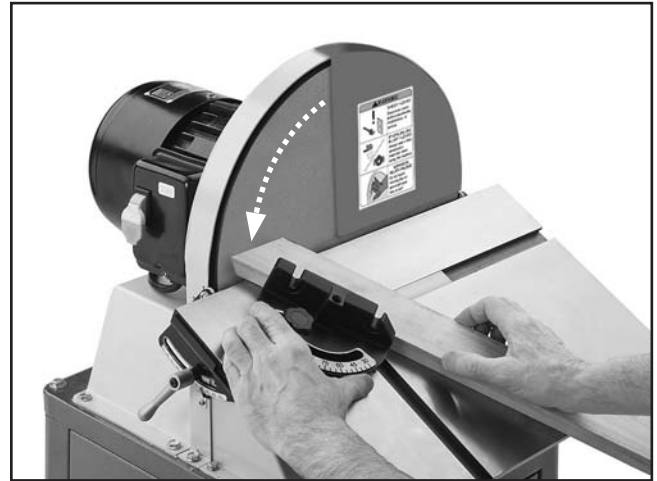
Figure 19. Sanding with table tilted.
