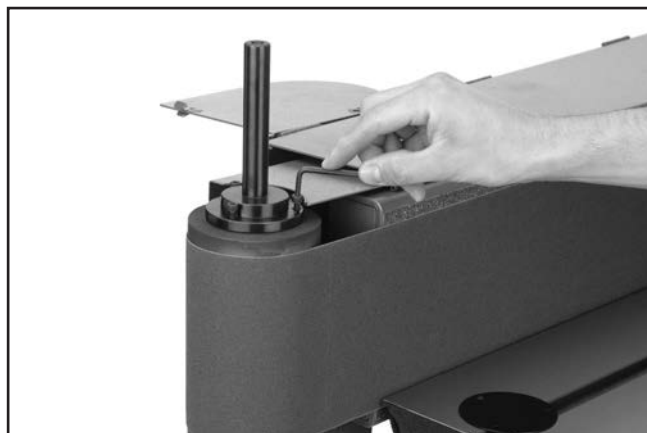
Figure 19. Tightening cap screws.
