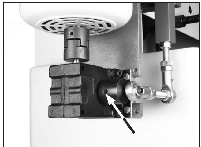
Figure 33. Eccentric set screw.
