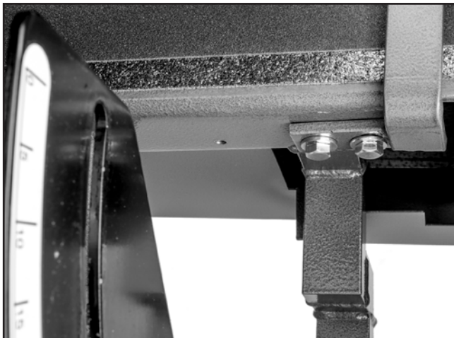
Figure 6. Back stop installed.
