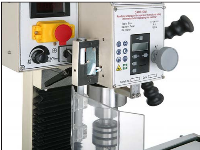
Figure 63. Chip guard limit switch.
