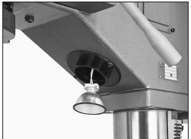
Figure 46. Work lamp wiring.
