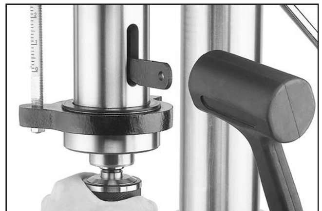
Figure 18. Using drift key to remove arbor.
