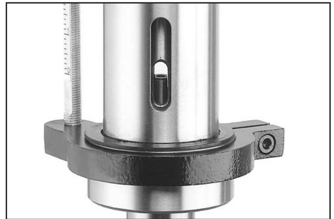
Figure 17. Spindle and quill drift key holes aligned.
