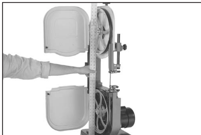
Figure 62. Checking if the wheels are coplanar.
