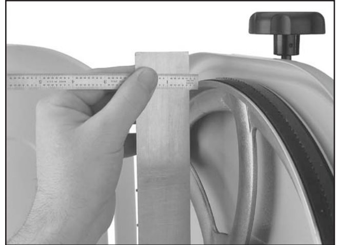
Figure 64. Measuring the distance to shim the wheel to be coplanar.
