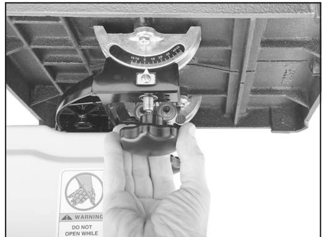
Figure 17. Securing table to the trunnion.
