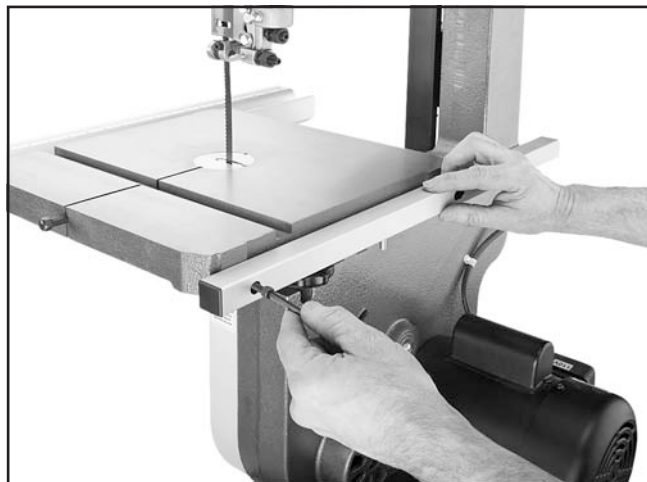
Figure 19. Attaching the rear fence rail.
