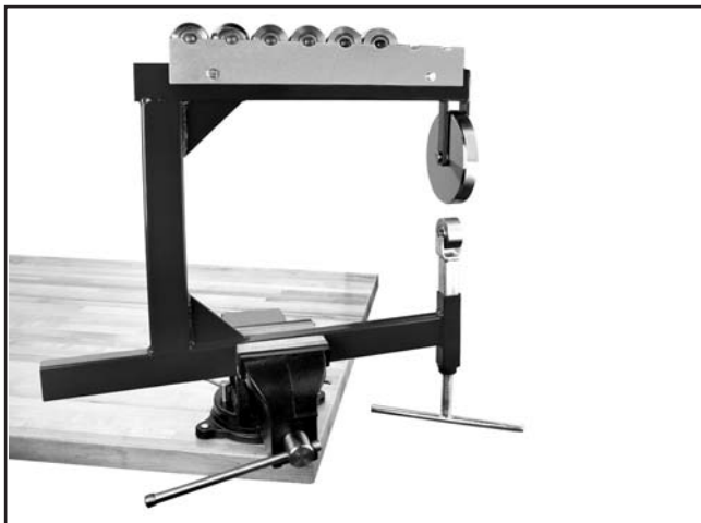
Figure 3. Example of Model T25101 secured in vise mounted to a workbench.
